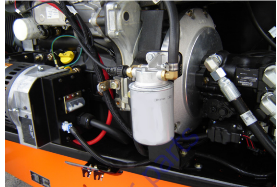
Figure 3-72. Location of the Primary Fuel Filter
