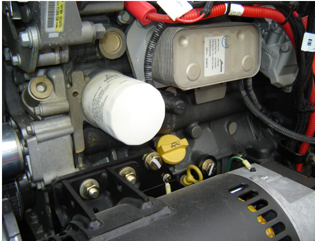
Figure 3-71. Location of the Oil Filter
