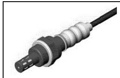
Figure 3-93. Heated Exhaust Gas Oxygen Sensor (HEGO)
