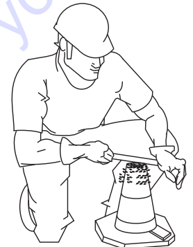
Figure 68-D. Slump Test (Removing Excess Concrete)
