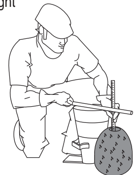
Figure 68-F. Slump Test (Measurement)
