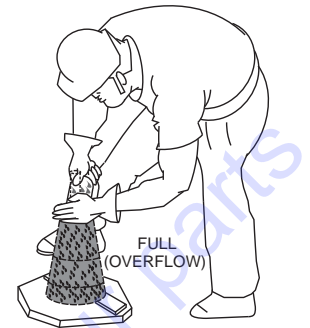
Figure 68-C. Slump Test (Full-Overflow)
