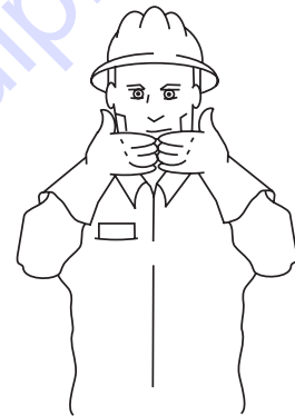
ALL DONE CLEAN-UP
