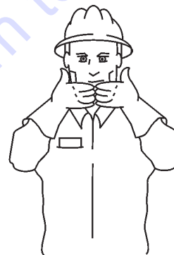
ALL DONE CLEAN-UP
