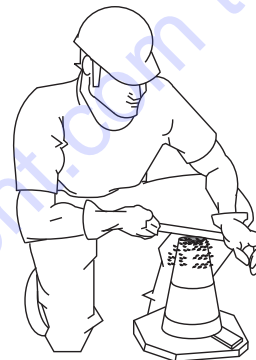
Figure 34-D. Slump Test (Removing Excess Concrete)
