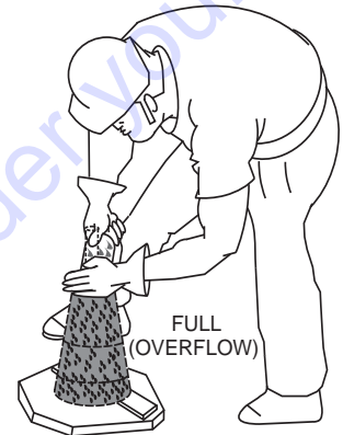
Figure 34-C. Slump Test (Full-Overflow)
