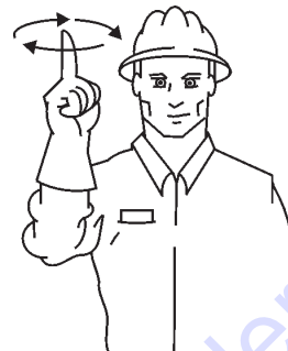
START PUMP SPEED UP
