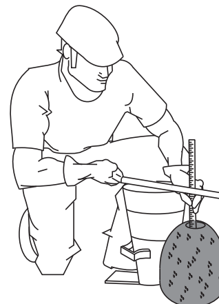
Figure 34-F. Slump Test (Measurement)
