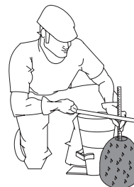
Figure S. Slump Test (Measurement)
