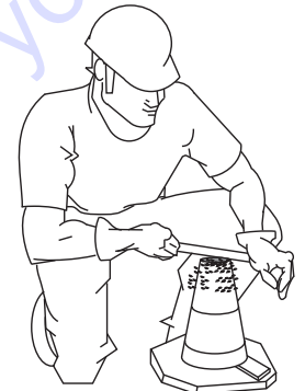
Figure 68-D. Slump Test (Removing Excess Concrete)
