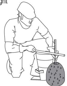
Figure 68-F. Slump Test (Measurement)
