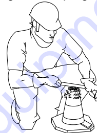
Figure Q. Slump Test (Removing Excess Concrete)
