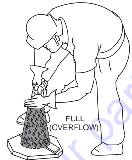
Figure 69-C. Slump Test (Full-Overflow)
