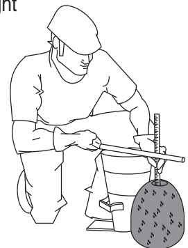
Figure 69-F. Slump Test (Measurement)
