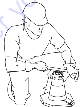
Figure 69-D. Slump Test (Removing Excess Concrete)
