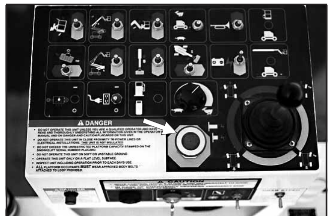
Platform control box Emergency Stop switch location.
