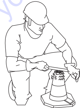
Figure 54-D. Slump Test (Removing Excess Concrete)
