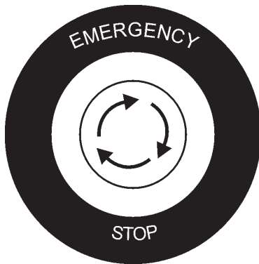
Figure 19. Emergency Stop Switch
