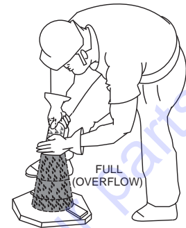
Figure 54-C. Slump Test (Full-Overflow)
