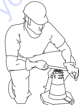
Figure 54-D. Slump Test (Removing Excess Concrete)
