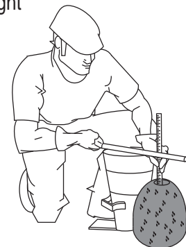
Figure 54-F. Slump Test (Measurement)
