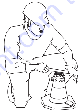
Figure 41-D. Slump Test (Removing Excess Concrete)
