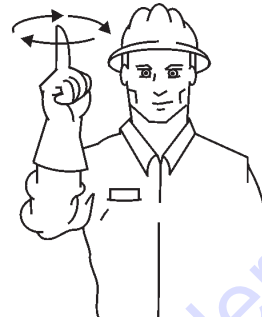
START PUMP SPEED UP
