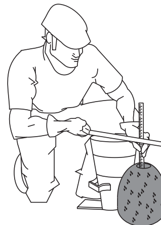
Figure 41-F. Slump Test (Measurement)
