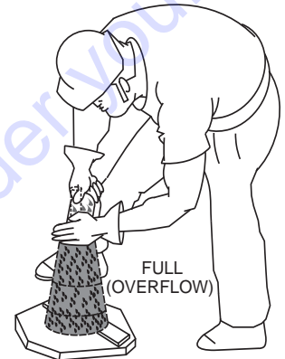
Figure 34-C. Slump Test (Full-Overflow)
