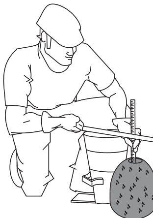
Figure 34-F. Slump Test (Measurement)
