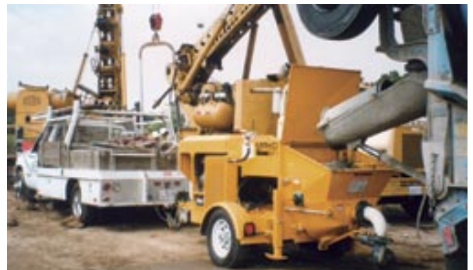
Drilling applications — Pumping up 80 feet and down 150 feet is easy for the Mayco LS-60.
