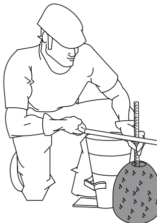
Figure 40-F. Slump Test (Measurement)
