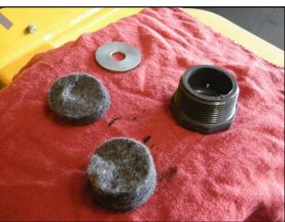
The cam rocker arm felt pads are part of maintenance and should be checked regularly.
