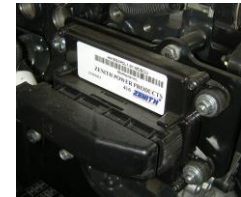
Engine Control Unit (ECU) Controls actuators via data from a series of sensors ensuring optimal eng. performance.
