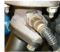
Oxygen Sensor 1/pre-cat (HO2S Sensor 1) Specifically used for controlling the air to fuel ratio of the engine.
