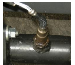
Oxygen Sensor 2/post-cat (HO2S Sensor 2) Specifically used for controlling the air to fuel ratio of the engine.
