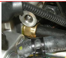
Water Temperature Sensor (Water Temp Sensor) The ECU adjusts various eng systems based on variable coolant temperature data.
