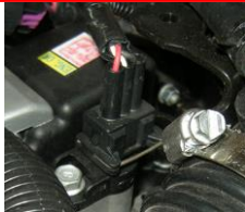
Top Dead Center/CAM Position Sensor (TDC/CMPS) CAM & CRANK positions data to ECU together derive the current combustion cycle.
