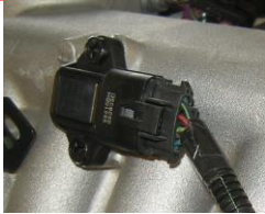
Manifold Absolute Pressure & Intake Air Temperature Sensor (MAP & IAT Sensor) Provides instant manifold pressure & temp information to the engine's ECU.
