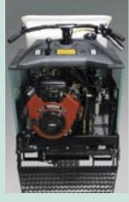
The operator can quickly change from standard drive to all wheel drive. This is ideal when used in adverse job conditions, greatly improving performance in sand, mud or loose gravel.
