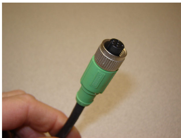
Figure 7-8. Phoenix Contact M12 – No Dielectric Grease
