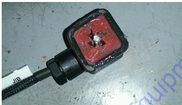
Figure 7-7. Brad-Harrison M12 – No Dielectric Grease
