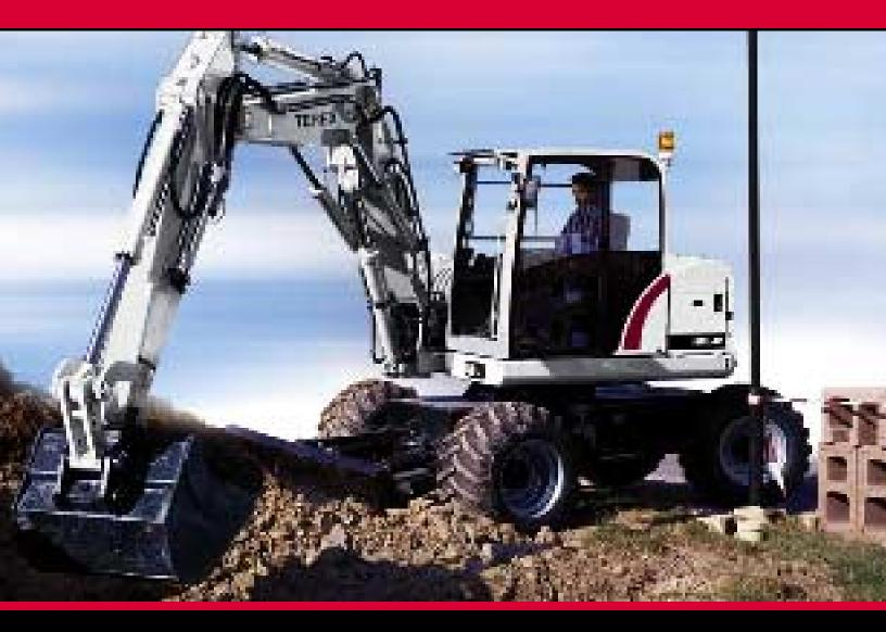
Infinitely variable speed Hydrostatic Drive Working hydraulic system independent of travel system Standard auxiliary hydraulic circuits Standard Quick-attach Large cabin design for "full size" operators Monoblock boom cylinder mounted on top for maximum protection Excellent maintenance access
