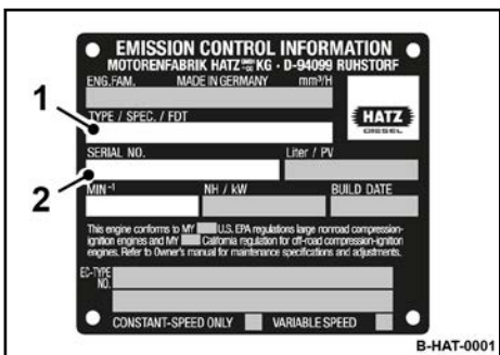
Fig. 2: Engine type plate (example)
