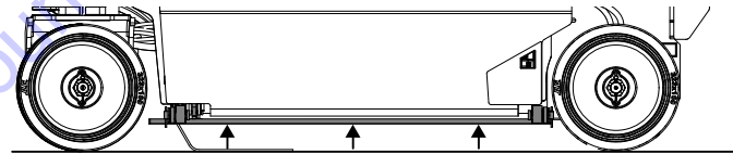
Platform Fully Lowered - Pothole Bars Raised
