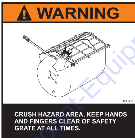
Figure 38. Safety Grate (Crush Hazard)
