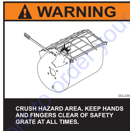
Figure 37. Safety Grate (Crush Hazard)
