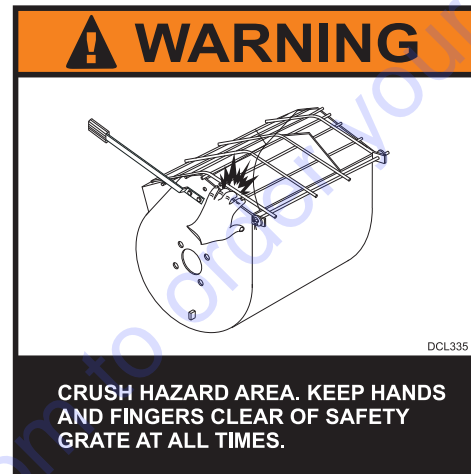
Figure 37. Safety Grate (Crush Hazard)
