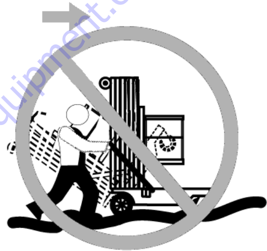
Figure 1-7. Do Not Move Unit on Soft or Uneven Surfaces or Over Obstructions, Bumps, Debris, Etc.
