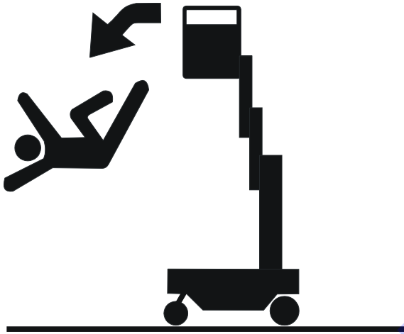
Figure 1-5. Falling from Platform could cause Death or Serious Injury.
