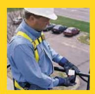
From their work platform, personnel can disable boom functions with access to the remote shutdown switch.
