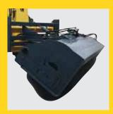
Mustang's Sweeper attachment, equipped with a hydraulic side-swing feature, keeps work surfaces clear of debris.
