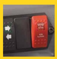
The WPS System is activated from the operator's station of the Mustang Telehandler.
