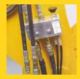
With Mustang Telehandler's circuit selector valve, only one set of auxiliary hydraulic hoses is required to operate both the hydraulic Quickattach II system and the hydraulically powered attachments.
