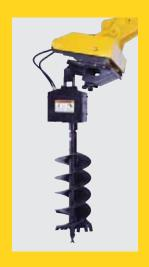
Attach a Mustang Auger to your Telehandler for fast hole drilling.
