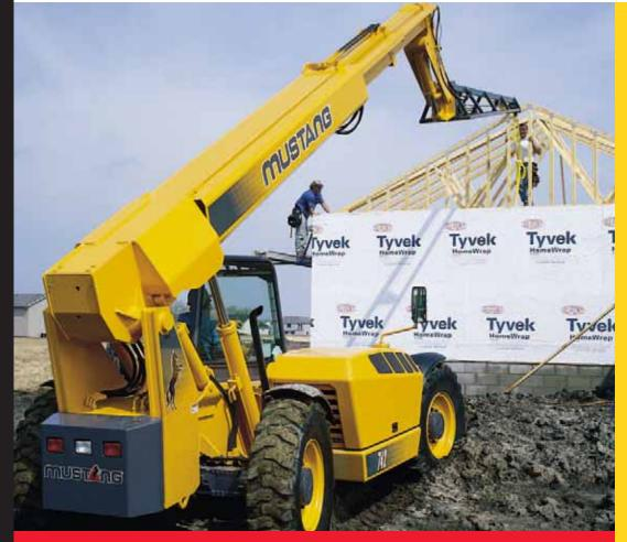
The Mustang Truss Boom gives operators the ability to position trusses with the utmost precision — up to four stories.
