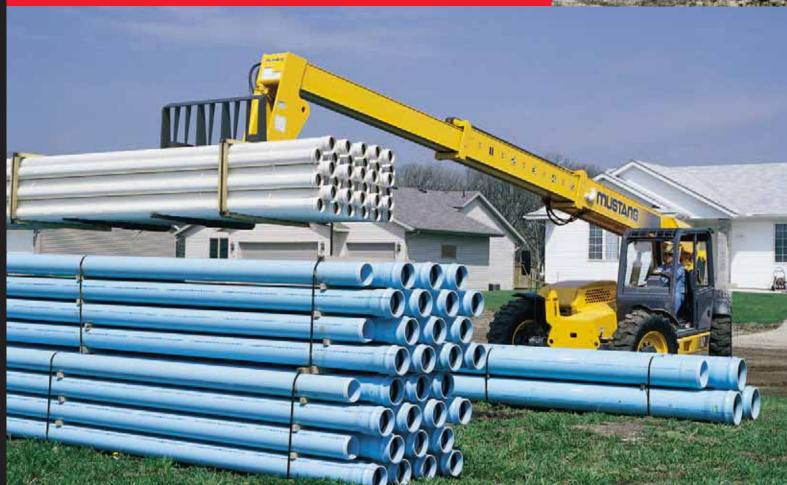
Getting into tight corners — and getting out — while moving loads through tough, muddy conditions on the job site is easy with a Mustang Telehandler. With a 146-inch outside turning radius, 20 degrees of frame tilt and three different steering modes, this large, heavy-duty machine becomes a nimble traveler. And with maximum forward reach of up to 40 feet, Mustang's Telehandler can overcome challenging obstacles and uncooperative terrain with ease.
