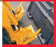
Multi-Tach™ mounting system allows for easy hookup of a wide variety of attachments. Compatible with most attachment systems in the industry.
