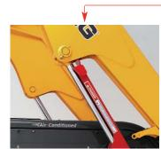
Lift arm support lock ensures positive lift arm locking in a raised position during maintenance and service.
