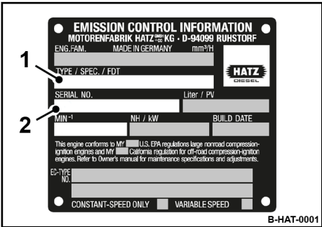
Fig. 2: Engine type plate (example)
