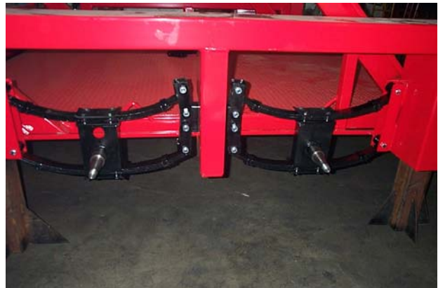
Figure 4-9. Dual, Quadra Spring Suspension
