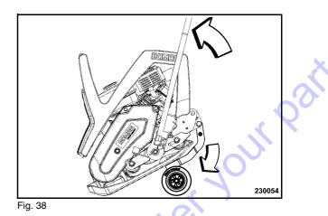
Push the vibratory plate up by the guide han-• dle (Fig. 38) and fold the transport wheels under the base plate.
