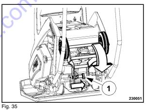
Unlock the safety bolt (1) (Fig. 35) and fold
