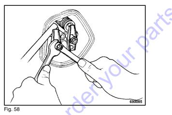
• Check the valve clearance with a feeler gauge on both valves (1) (Fig. 58).
