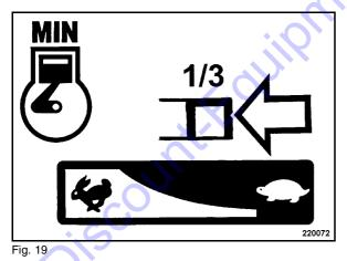
• Set the throttle lever (Fig. 19) to 1/3 throttle position.
