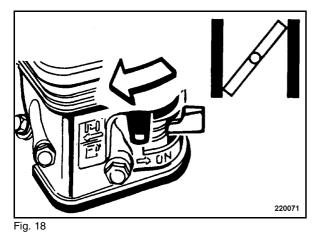
• Close the choke completely by shifting the lever (Fig. 18) in direction of arrow against the end stop.
