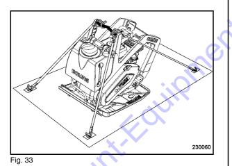
• Tie the machine to the transport vehicle, fasten the lashing gear to the cross-bar (Fig. 33) on the machine. Transport wheels<sup>\*</sup> with guide handle at rear.
