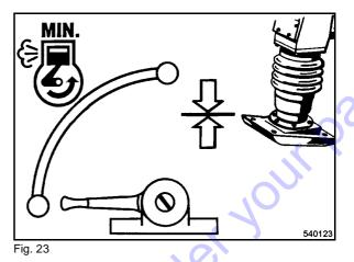
• During short breaks you should always set the throttle lever to "MIN"-position (Fig. 23).
