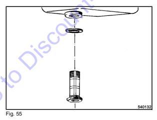
• Screw the strainer (Fig. 55) out and clean it with gasoline.
