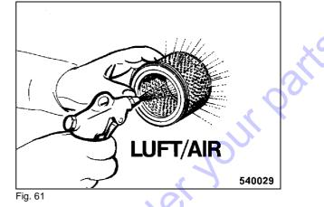
In case of dry fine dust blow out the filter cartridge carefully from inside to outside with dry, clean compressed air (Fig. 61) (max. 6 bar).
