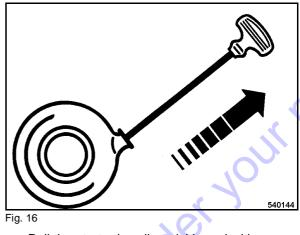
• Pull the starter handle quickly and with power (Fig. 16).
