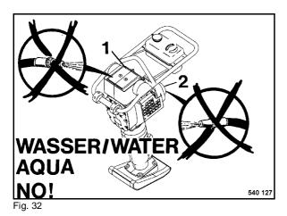
Do not guide the water jet directly into the air filter 1 (Fig. 32) and into the starter/air intake (2).
