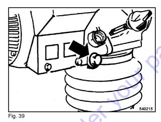
• Unscrew the drain plug (Fig. 39).
