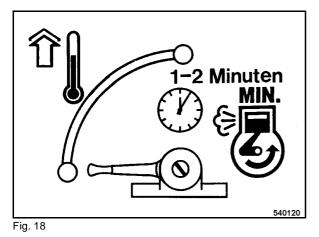
• Set the throttle lever (Fig. 18) to "MIN" and let the engine run warm for 1 to 2 minutes.
