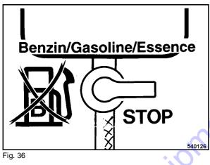
• Set the fuel valve (Fig. 36) to STOP position (closed).
