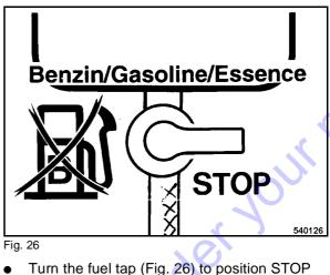
Turn the fuel tap (Fig. 26) to position STOP (closed).
