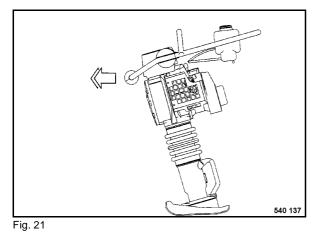
• The travel speed can be influenced by altering the load on the steering handle (Fig. 21).
