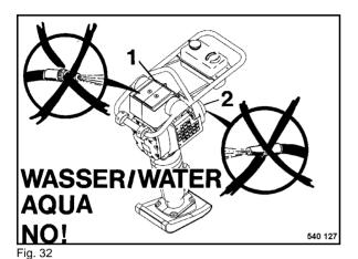
Do not guide the water jet directly into the air filter 1 (Fig. 32) and into the starter/air intake (2).
