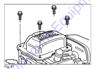
Unscrew the fastening screws for the cylinder head cover (Fig. 47).
