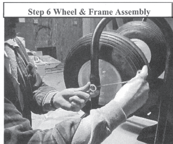
Place lock collars on axle shaft and tighten with Allen Wrench.
