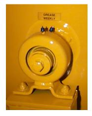
C. Always grease drum seals (both ends as recommended in the maintenance chart. The grease purges dirt--prolonging bearing life.
