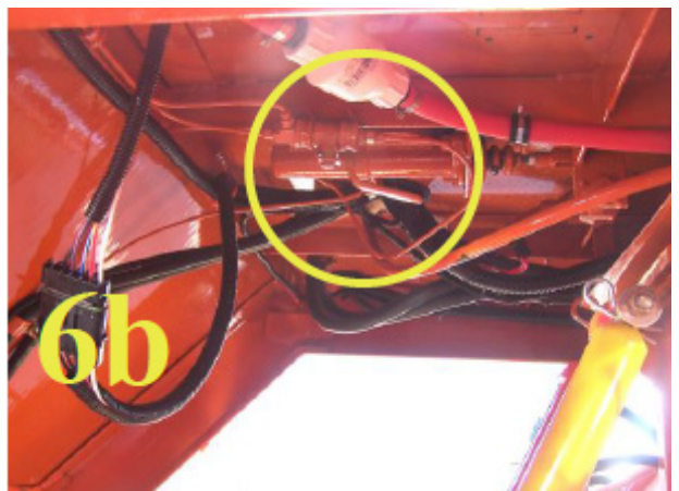
Surge brake only - close valve for towing (valve open in photo)
