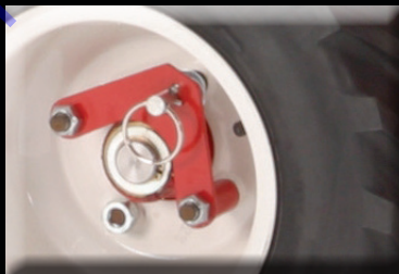
Hubs unlock to free-wheel the tiller when the engine isn't running
