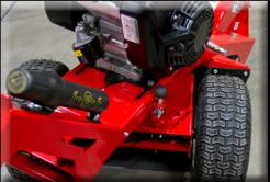
The innovative pivot over center swivel head design allows the grinding wheel to sweep easily across the stump.
