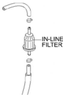
Figure 12. In-Line Fuel Filter
