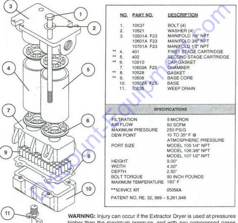
**WARNING:** Injury can occur if the Extractor Dryer is used at pressures higher than the maximum pressure, and with any compressed gases other than normal compressed air for power tool use only.
