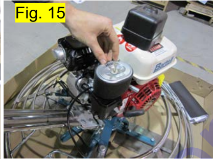
Step 12: Reinstall air filter and cover (Fig. 15)
