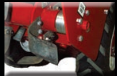
Counter-rotating tines cut through sod and hard packed soil
