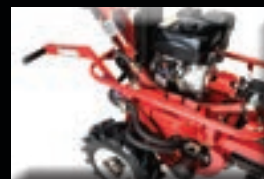
Manual lever lowers the boom and locks in one of three positions for trench depth
