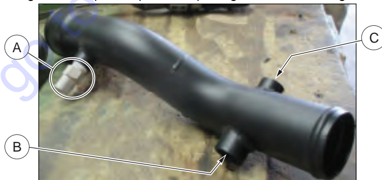
Figure 7 - Fitting and Cord Grip Locations
