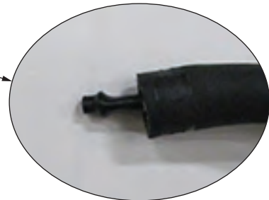
Figure 12 - Heat Cable Through PCV Hose—No Yellow Visible
