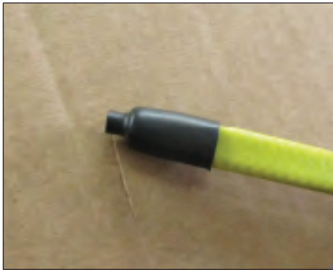
Figure 11 - Shrink End-Cap to Cable
