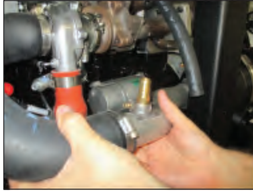
Figure 4 - Detaching Hoses, Removing Weldment
