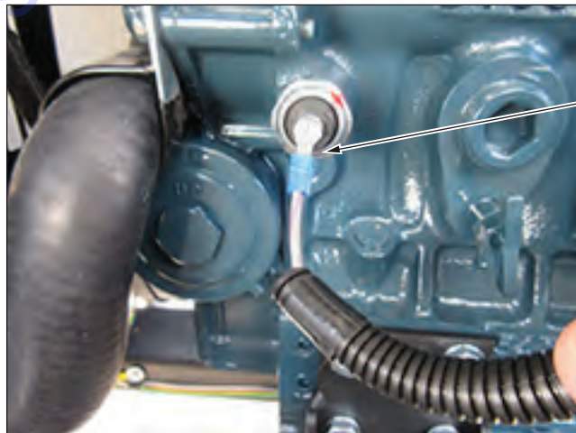
Figure 30 - Connect Oil Pressure Switch Wire
