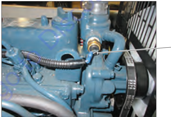
Figure 4 - Coolant Temperature Sensor Wire (Top of Engine)
