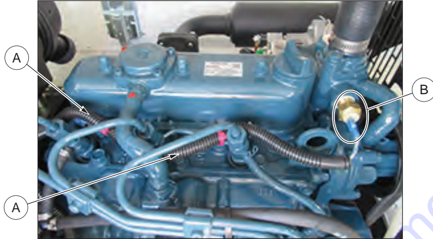
Figure 26 - Route Gray/Blue Wire to Coolant Temperature Switch
