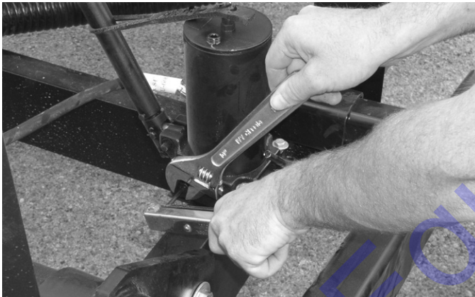
Figure B21 Adjusting Hydraulic Pump Bypass
