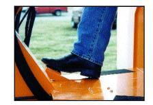
Wide, no-slip honeycomb surface provides less operator fatigue and improved operational comfort.
