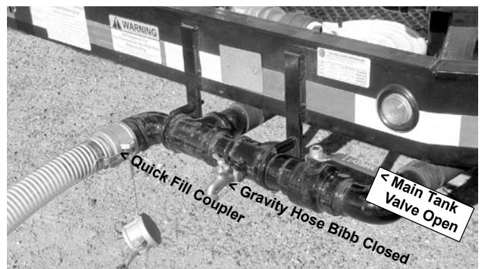
Figure B4 Filling Tank With Transfer Pump
