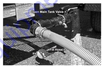
Figure B28 Filling Through Suction Manifold (500/800 Gal.)
