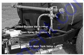
Figure B32 Spray Bar Valve/Bypass Valve Setting
