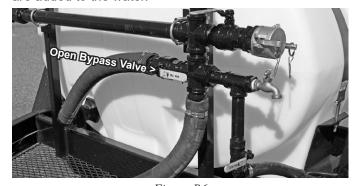
Figure B6 Open Bypass Valve
