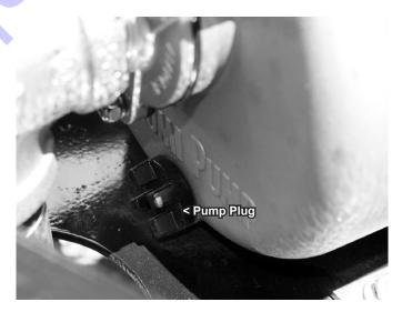
Figure C2 Pump Drain Plug
