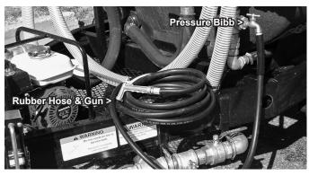
Figure B38 Rubber Hose on Pressure Bibb
