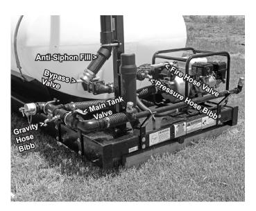
Figure B2 Water Skid Valves
