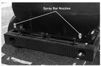
Figure B33 Spray Bar Nozzles (500 Gal.)
