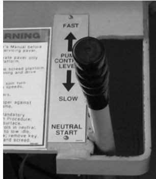
NOTE: Variable-Speed Control Lever Shown in Neutral Position
