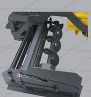
Independent hydraulically driven augers found on the screed extensions on the 1648 model are efficient at moving material to the end of the extension, allowing for a true 13 foot paving experience.
