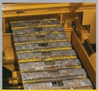
The direct-drive track design is self-cleaning and adjusts tension with a hydraulic cylinder. The track design is resistant to slipping, providing versatility in different sub-base conditions.
